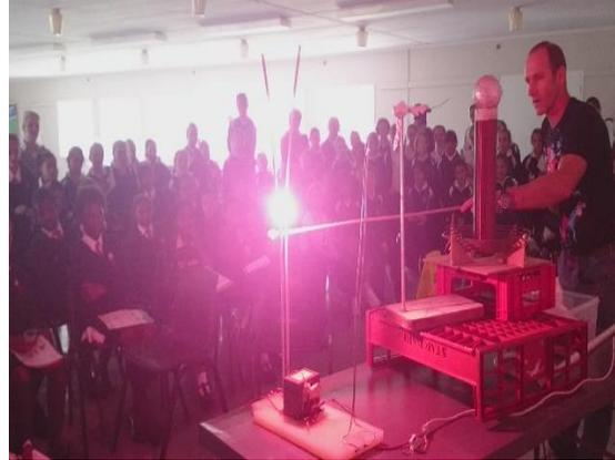
Making an arc red with strontium – this element is used in distress flares.
