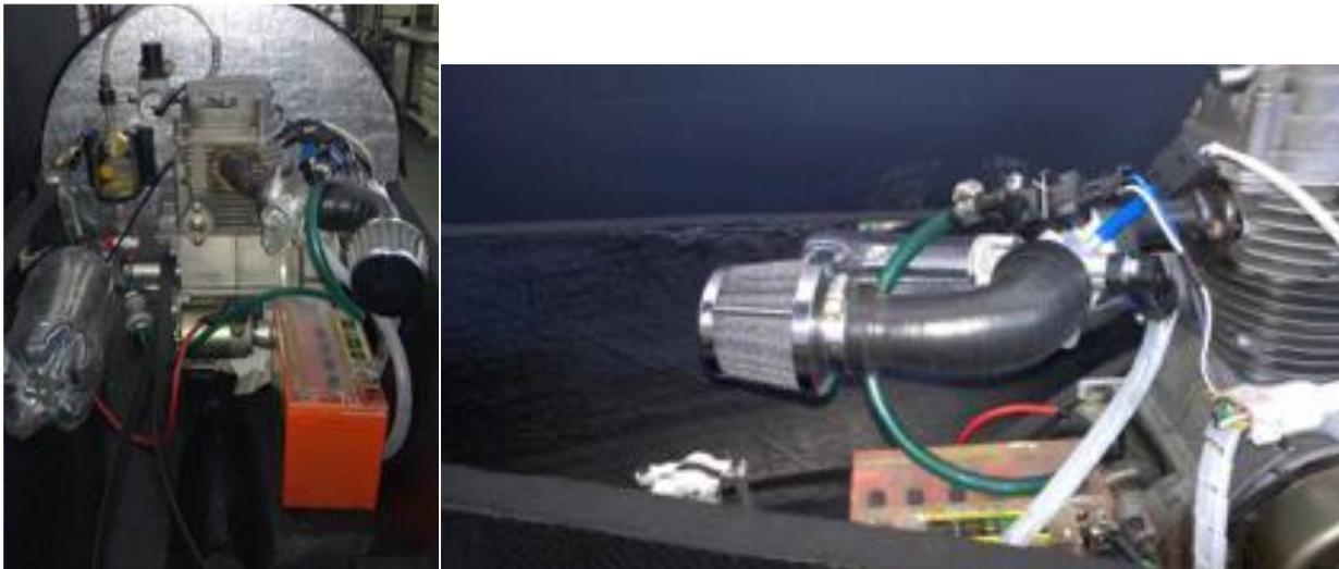
Thermal protection and mounted lines, wires and components (left). Manufactured air intake manifold with air intake filter fitted (right)
