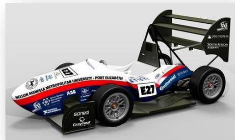
NMMU Racing has produced two vehicles in the combustion engine category, of which one competed successfully at the German Formula Student event in 2011. An electric vehicle is also under development which features a brushless-DC electric motor, a 400V battery pack and a self-design battery management system based on the National Instruments Compact Rio architecture.
